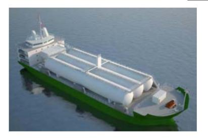
Proposed LNG Bunker Barge design: This design uses 3 x IMO Type-C LNG tanks, each with a capacity of 32,820 Cu.Ft. water volume. 3 x LNG Cargo Deep Well Pumps and suitable Boil-Off controls as per vendor requirement. Propelled by 2 x ASD Thrusters and 3 x Diesel Driven Alternators. Design for alternative Classification Society, Crew strength, propulsion power others can be made. Details available immediately upon request.
